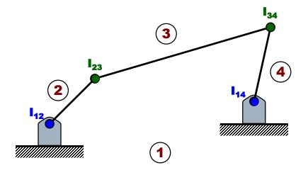
Need to locate the SECONDARY Instant Centers  $I_{13}$  and  $I_{24}$
