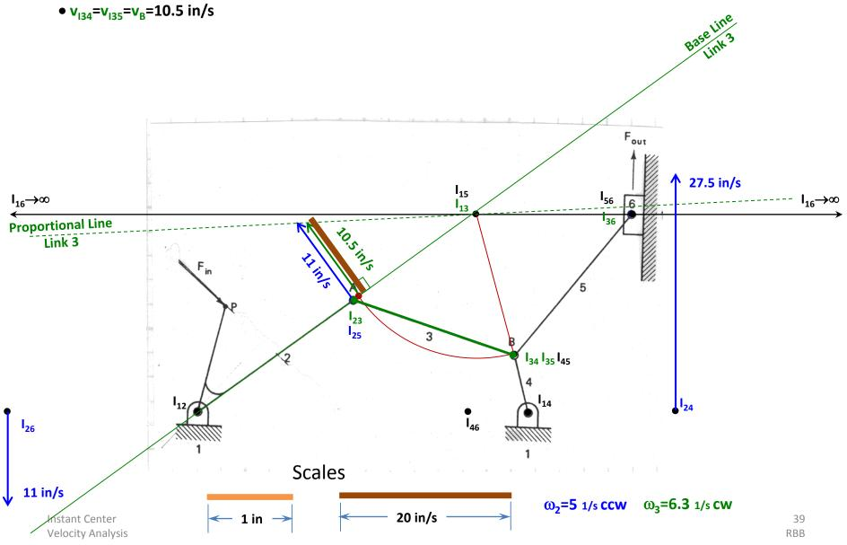
Starting by finding the LINEAR VELOCITIES of Instant Centers I<sub>34</sub>, and I<sub>35</sub>
