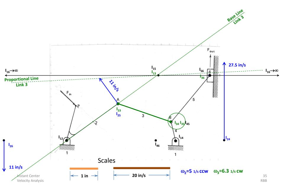
Starting by finding the LINEAR VELOCITIES of Instant Centers I<sub>34</sub>, and I<sub>35</sub>
