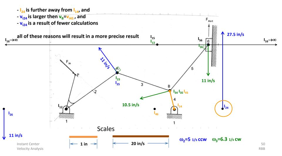
At this instant, Link 4 appears to be rotating, with respect to the ground (Link 1), about Instant Center  $I_{14}$ A known velocity on Link 4 is  $v_{124}$ =27.5 in/s
