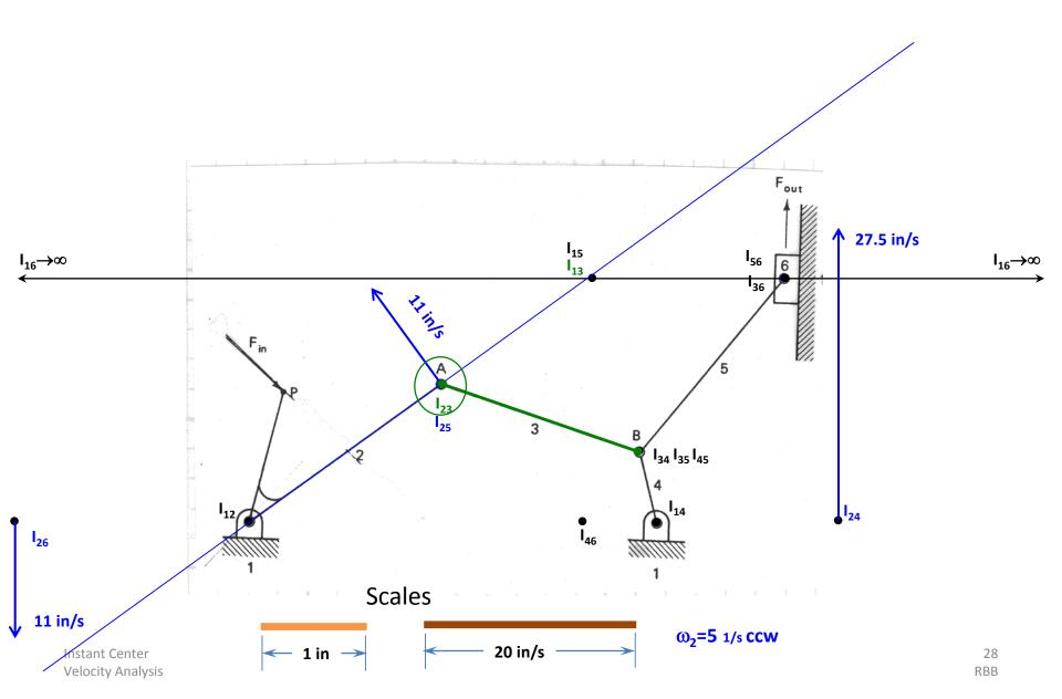
At this instant, Link 3 appears to be rotating, with respect to the ground (Link 1), about Instant Center  $I_{13}$ A known velocity on Link 3 is at A which is the same as  $I_{23}$ ,  $v_A = v_{123} = 11$  in/s
