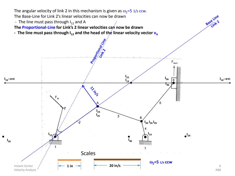
The velocity of any point on Link 2 can now be determined by scribing an arc centered at  $I_{12}$ , from the point of interest on Link 2 to the Link 2 Base Line. The linear velocity vector is then determined by drawing a line perpendicular to the Base Line out to the Proportional Line. The scaled distance is the linear velocity of the point.
