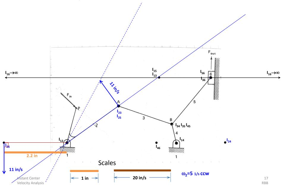
An ALTERNATE approach to determining the Linear Velocity of Instant Center I<sub>26</sub>
