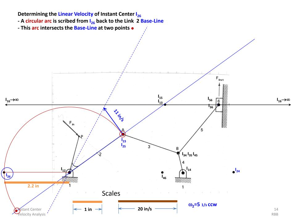
Determining the Linear Velocity of Instant Center I<sub>26</sub>
