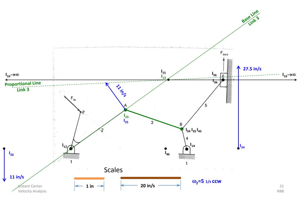
The angular velocity of Link 3,  $\omega_3$ , can now be calculated - The distance from I<sub>13</sub> to A/I<sub>23</sub> is measured, r<sub>I13I23</sub>=1.75 in
