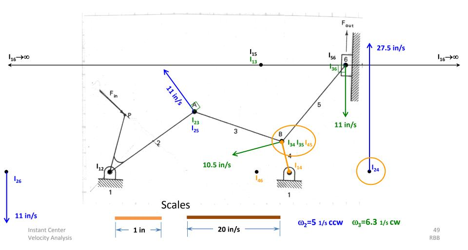
At this instant, Link 4 appears to be rotating, with respect to the ground (Link 1), about Instant Center I14
