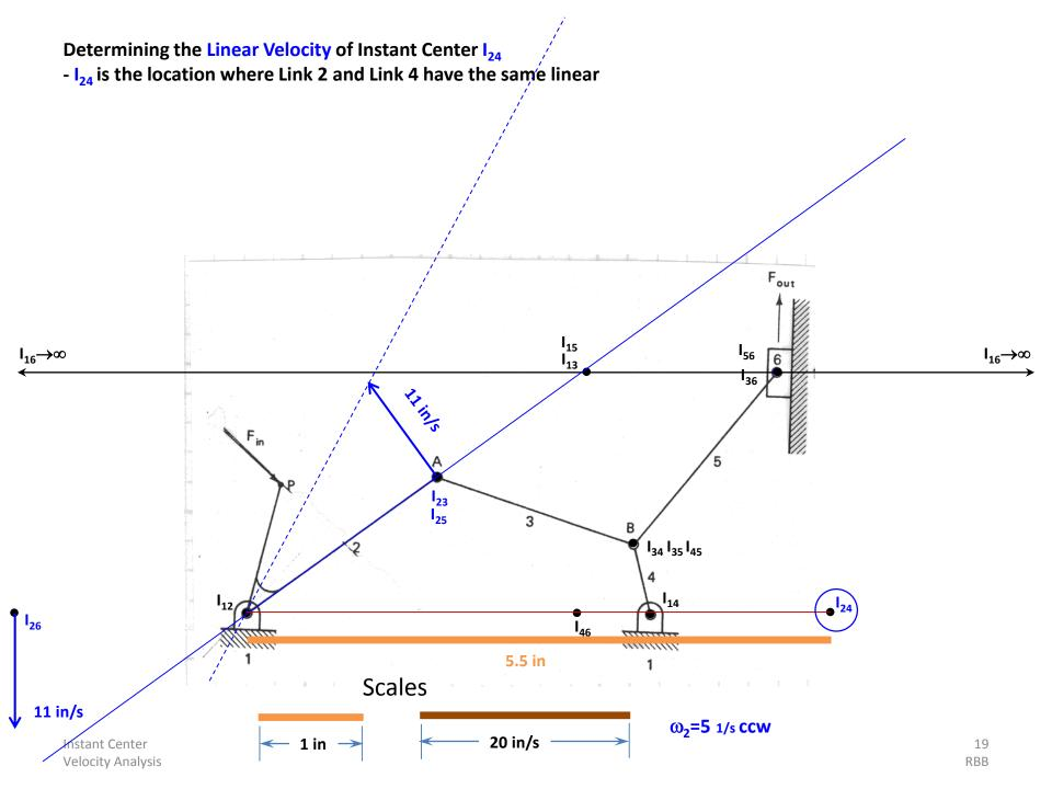
Determining the Linear Velocity of Instant Center I24
