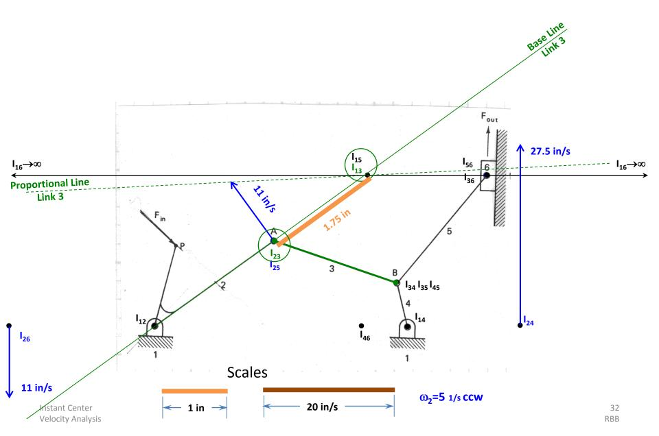
The angular velocity of Link 3,  $\omega_3$ , can now be calculated
