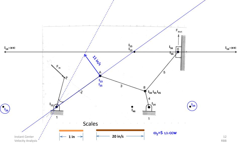
Determining the Linear Velocity of Instant Center I<sub>26</sub> - I<sub>26</sub> is the location on Link 2 where the linear velocity is the same as on Link 6
