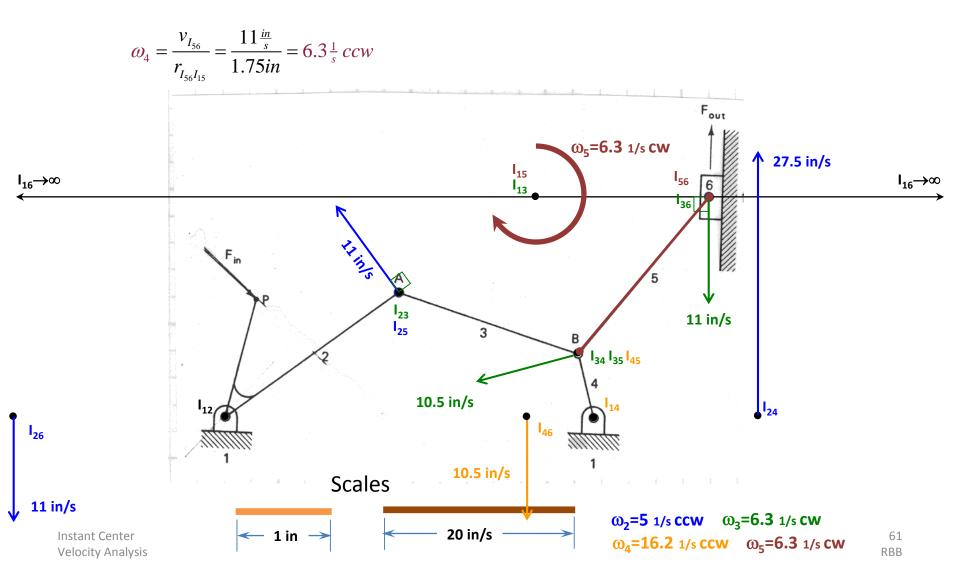
All LINEAR VELOCITIES of the INSTANT CENTERS and all the ANGULAR VELOCITIES of this mechanism have been determined. The diagram below illustrates the instant center solution to his problem.
