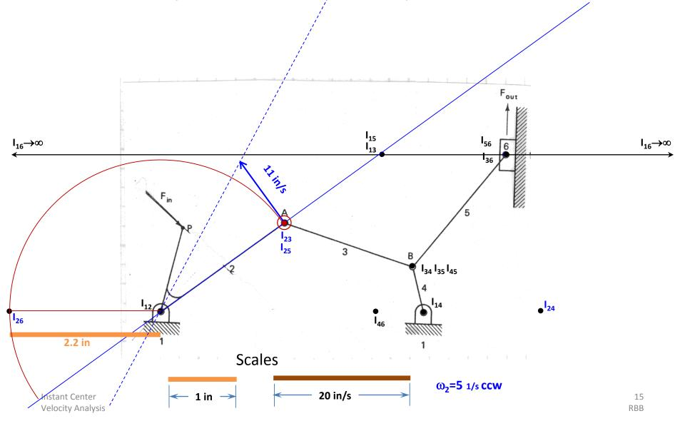
Determining the Linear Velocity of Instant Center I<sub>26</sub>
