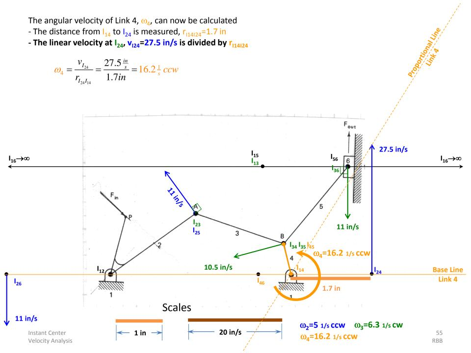
The angular velocity of Link 4,  $\omega_4$ , could ALTERNATELY be calculated using
