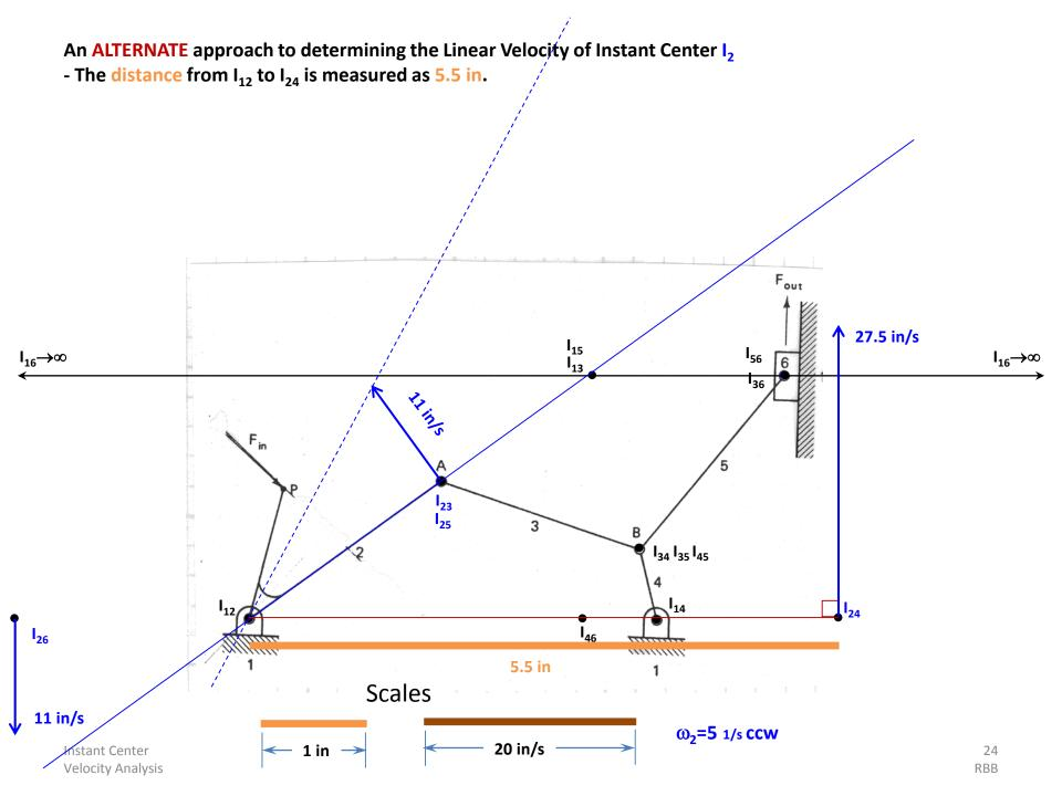
An ALTERNATE approach to determining the Linear Velocity of Instant Center  ${\rm I_2}$
