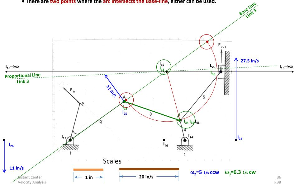
Starting by finding the LINEAR VELOCITIES of Instant Centers I<sub>34</sub>, and I<sub>35</sub> Instant Centers  $I_{34}$ , and  $I_{35}$  are both at point B
