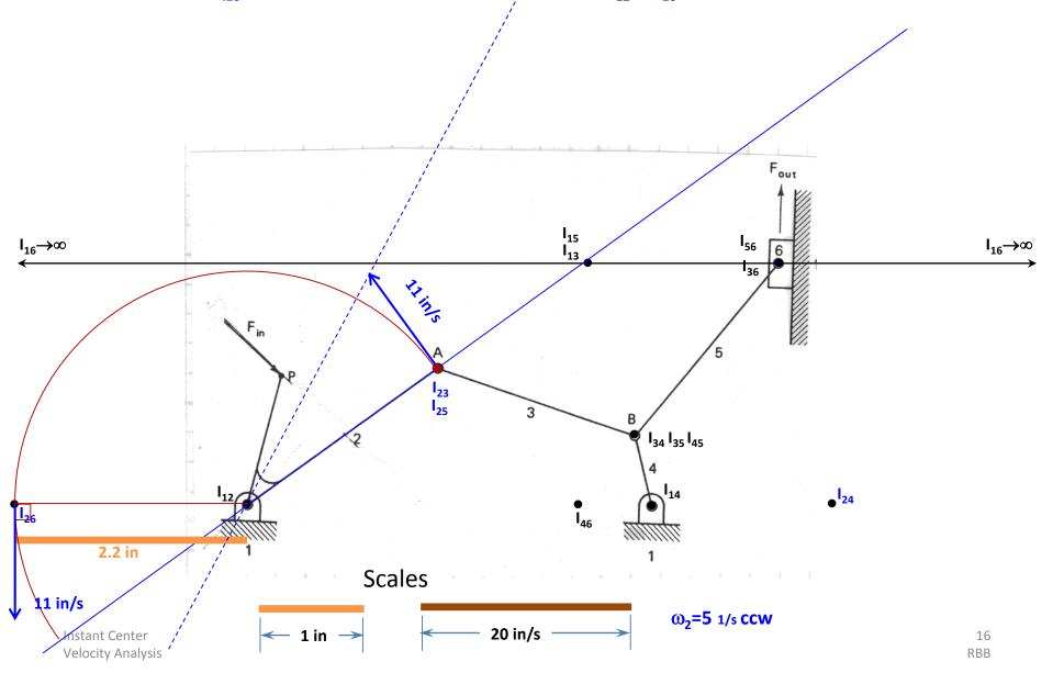
An ALTERNATE approach to determining the Linear Velocity of Instant Center  ${\rm I_{26}}$
