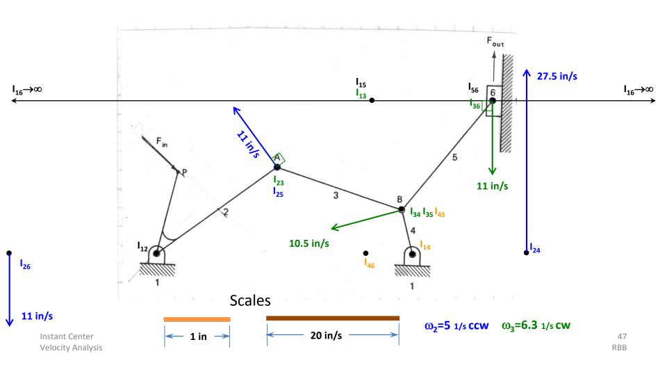
At this instant, Link 4 appears to be rotating, with respect to the ground (Link 1), about Instant Center I<sub>14</sub>
