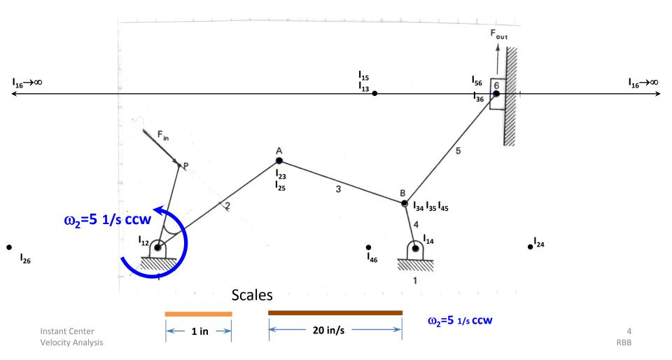
The angular velocity of link 2 in this mechanism is given as  $\omega_2=5 \text{ 1/s ccw}$ .
