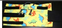
Figure 1: Air bladder inside a fabric cover which will wrap around the stump
