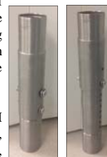
Figure 6: Images of the pylon prototype at its shortest height, slot A (left), and its tallest height, slot I (right)
